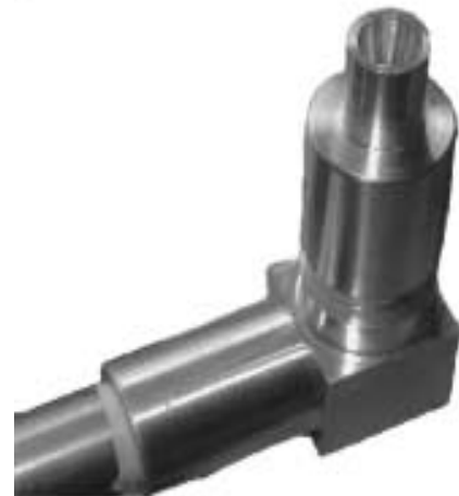
Close up of test thruster attached to test set up.
