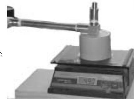
Cold gas thrust chamber being tested.
