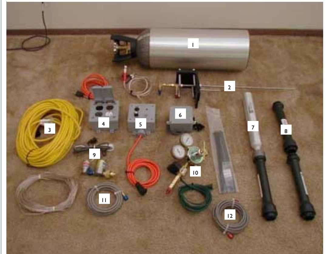
(1) N2O Storage tank, (2) Fill stem assembly, (3) Control cable, (4) Launch pad junction box, (5) Launch control box, (6), (7) N2O Tank, (8) Fuel grain, (9) N2O and GOX solenoid assemblies, (10) Gas regulator, (11) N2O Hose, (12) GOX Hose
